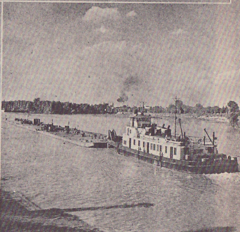
9. This type has practically edged out the sternwheelers—the all-metal, screw Diesel. A survey of postwar planning has shown that almost all river vessels now on the drawing boards are propeller-equipped.
