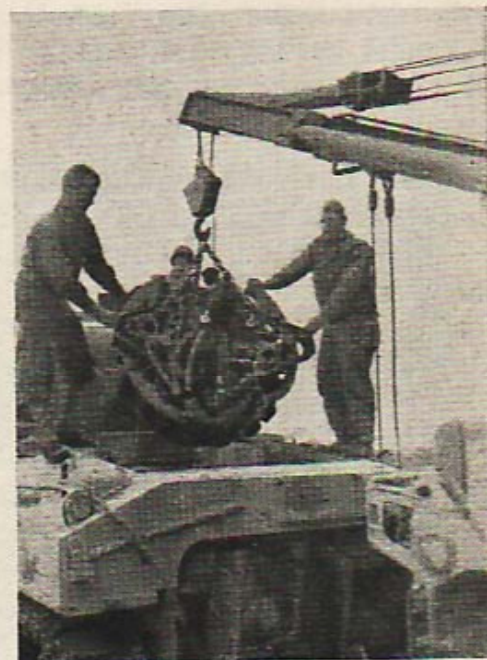
Maintenance men of the 129th Ord Bn replace an engine in a battleworn tank of the Division.
