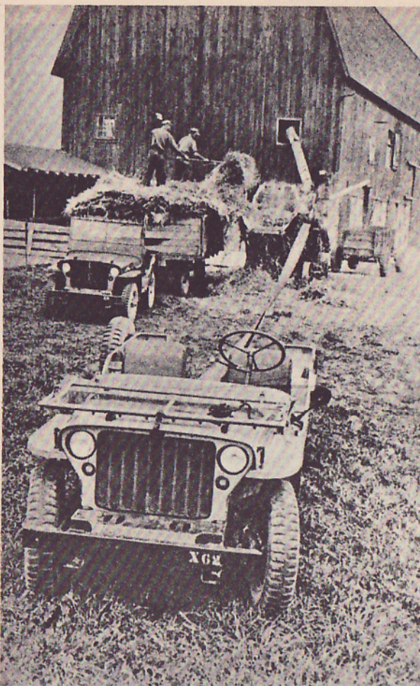
CIVVY JEEPS. THESE BUGGIES AREN'T WAR VETERANS WITH 85 POINTS. THEY'RE NEW ONES DEVELOPED BY WILLYS-OVERLAND, AND HERE THEY ARE OPERATING AS PORTABLE POWER UNITS TO RUN A THRESHING MACHINE.
